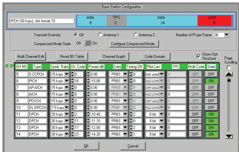
Definition of a code channel scenario for WCDMA 3GPP FDD mode
